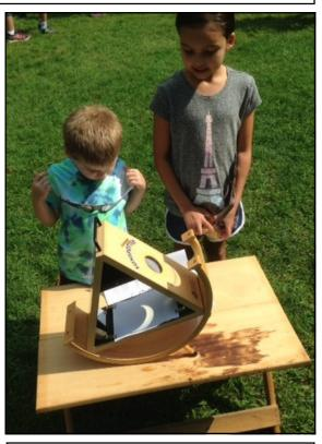
Mary Lou West's Sunspotter was a big hit at the NJAG event at the Haworth Public Library. By using a series of mirrors, the device projects a solar image onto a viewing screen through a powerful 62mm diameter objective lens. photo by Mark Zdziarski
